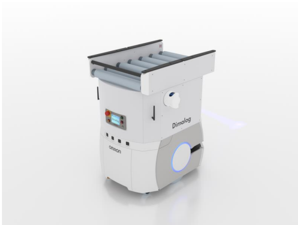
Roller Conveyor LD-60/90-RC-LW-2 with Integration Module IM7L.
