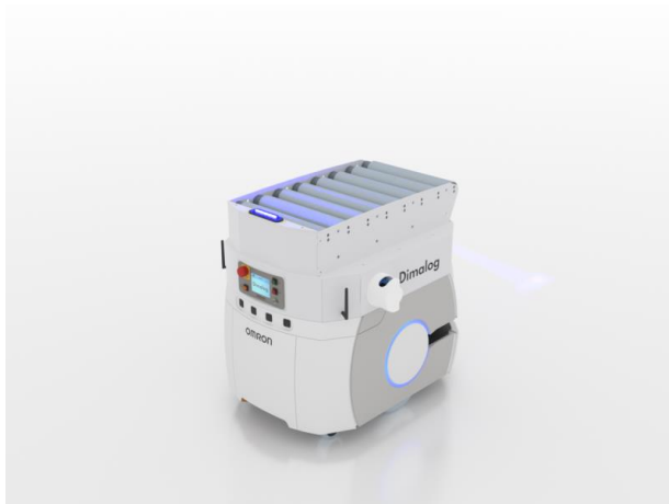
Light Roller Conveyor RC-LT-1 with Integration Module IM5L.
